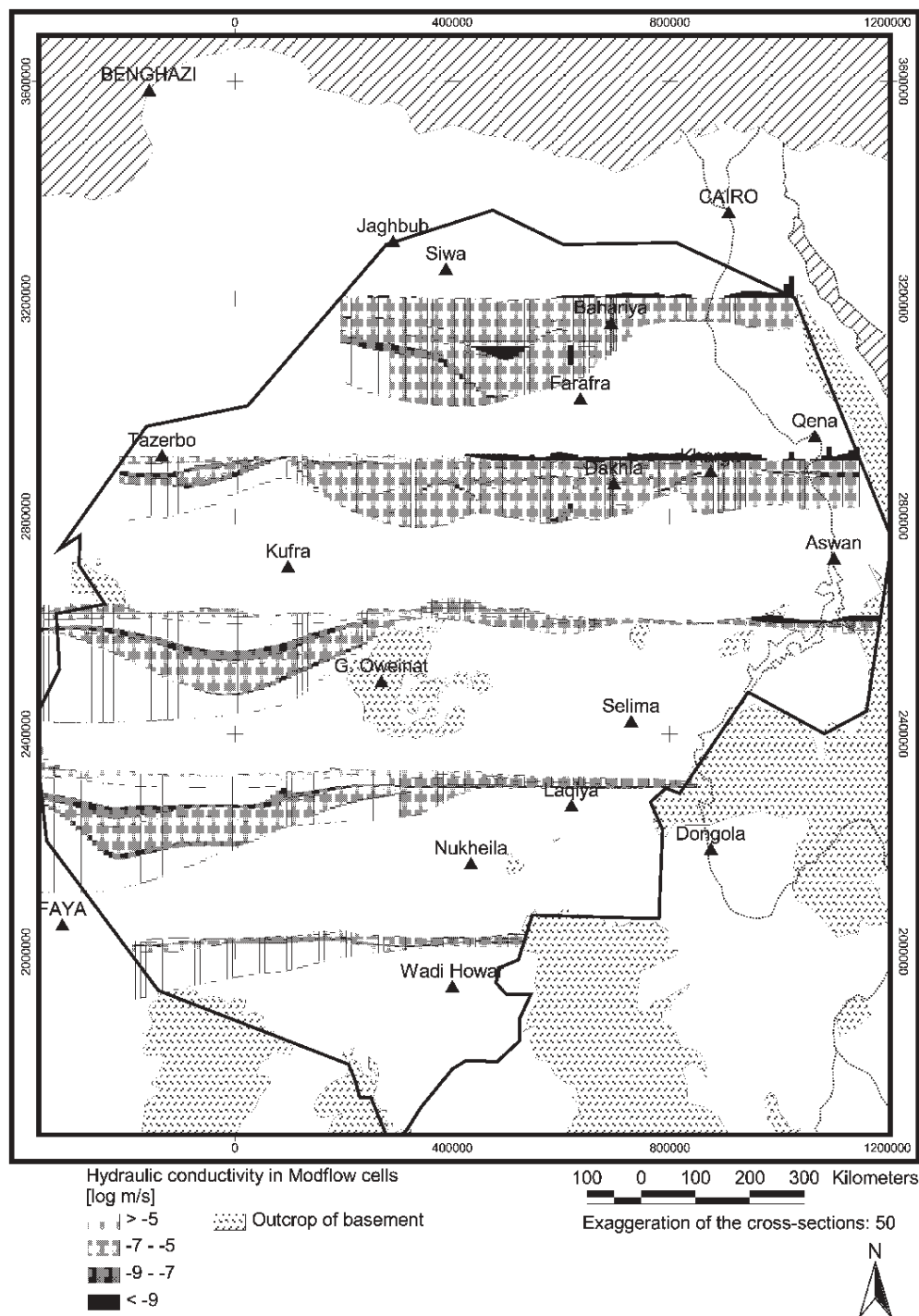
Fig. 3 Cross sections of hydraulic conductivities for the Nubian Aquifer System as they are implemented in the numerical groundwater model
