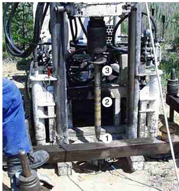
Fig. 1. Cone Penetration Test (CPT) equipment (Elgoscarr 2000 Ltd.) used at Krauthausen test site: 1. cone penetrometer, 2. three electrodes, 3. hollow push rods.
