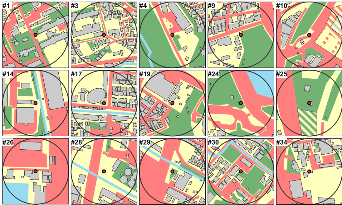
Fig. 2. Buildings (grey) and land cover around all well locations (red dot). Land covered by asphalt such as streets or parking lots are depicted in red, land covered by grass is green and water is given in blue. Within this study buildings and land cover types within a radius of up to of 100 m (black circle) are considered. For wells #10 and #25 areas affected by the land cover changes in 2007 are framed with a thin grey line and shown in striped colors. (For interpretation of the references to color in this figure legend, the reader is referred to the web version of this article.)
