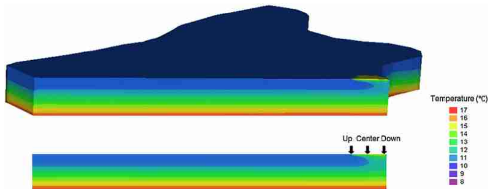
Figure 5. Temperature distribution after 110 years simulation (reference case with linear temperature increase at hot spot) for selected cross-section of 3D model and of emulated vertical 2D model; 'center' indicates the city centre and 'down' is near river Rhine
