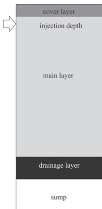
Figure 1. Vertical flow filter schematic cross section—the arrow indicates the injection depth of Scenario 2 (base case).
